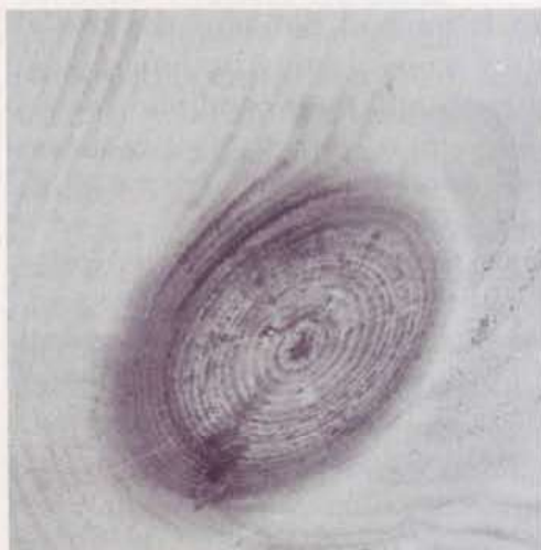
Sound, tight (intergrown), oval red knot.
